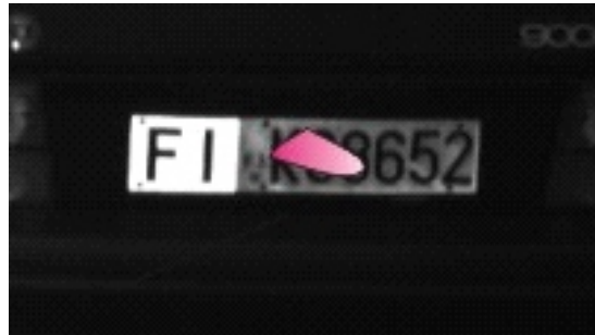
B) Reflective surface corroded or defective
