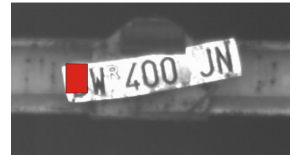
C) Plate mounted incorrectly
